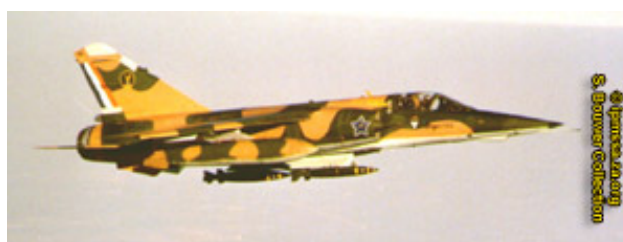
F1 AZ with 4 Mk 81 bombs and two under wing fuel tanks. This configuration was typical during the early deployment to the operational area.
