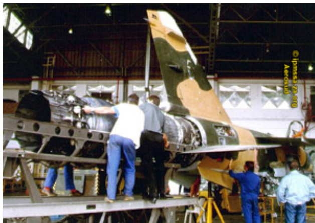
The SMR-95 engine being installed in AZ No 216, by AEROSUD.
