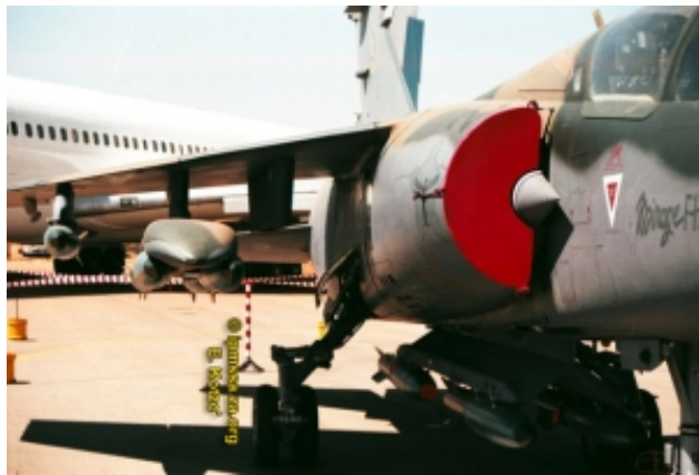
The latest underwing bomb rack as used in the 14 bomb configuration, use a underwing bomb dispenser unit, with integral fuel tank. Only the AZ carried this type of dispenser.
