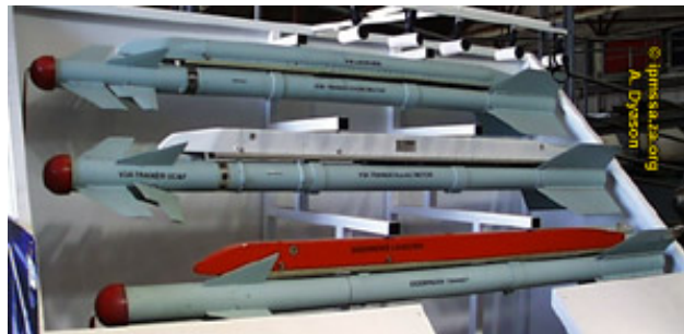
V3B top, V3A middle, AIM 9B bottom. Note: different launcher rails.
