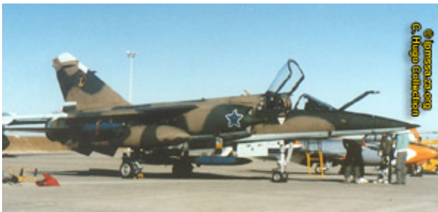
F1 AZ with under wing auxiliary fuel tanks. This could also be fitted to the CZ. This is another typical Border War configuration - 6x iron bombs, 2x underwing fuel tanks and 2x V3B missiles.
